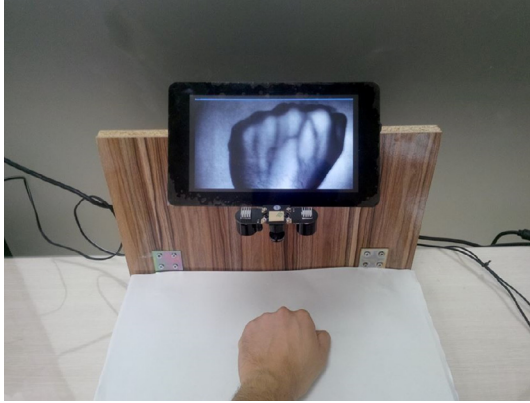
Fig. 2.6. Data acquisition procedure of the vein-pattern imaging system.
