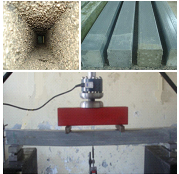
Fig. 2. Hybrid beams and flexure test.
