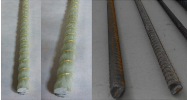
Fig. 5. FRP and Steel Bars
