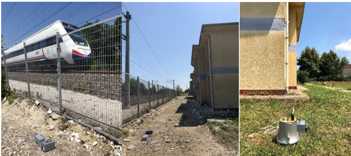
Figure 2 Field view and accelerometer locations
