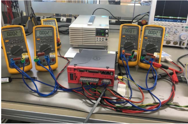
Fig. 2. Test setup for measuring motor currents.
