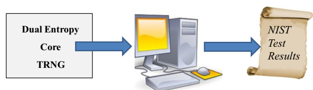
Fig. 8 The designed structure for testing the randomness of generated data set obtained from TRNG unit
