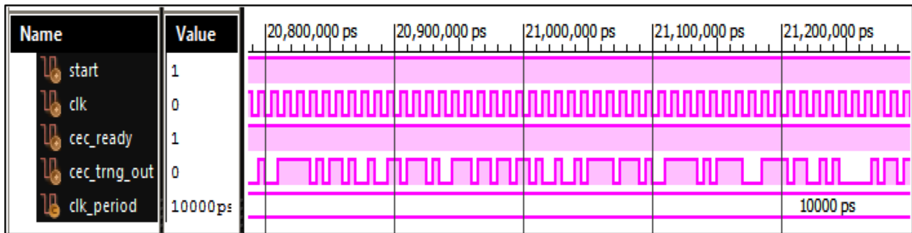
Fig. 7 Xilinx ISE simulator result of the designed dual entropy core new TRNG unit
