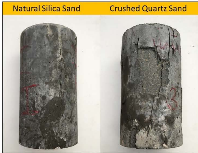
Fig. 15. View of the specimens after compression test.
