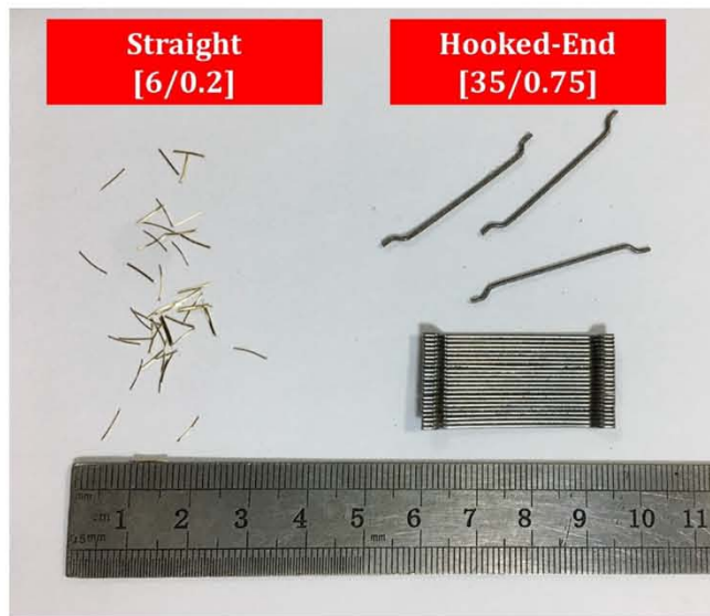
Fig. 1. Types of steel fibers used in the study.
