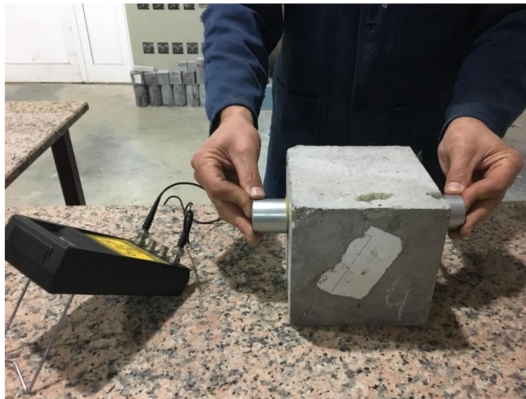
Fig. 4 - Sound pulse velocity experimental setup
