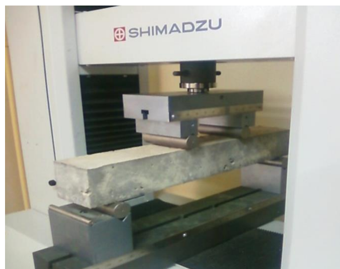
Fig. 3 - Flexural test apparatus
