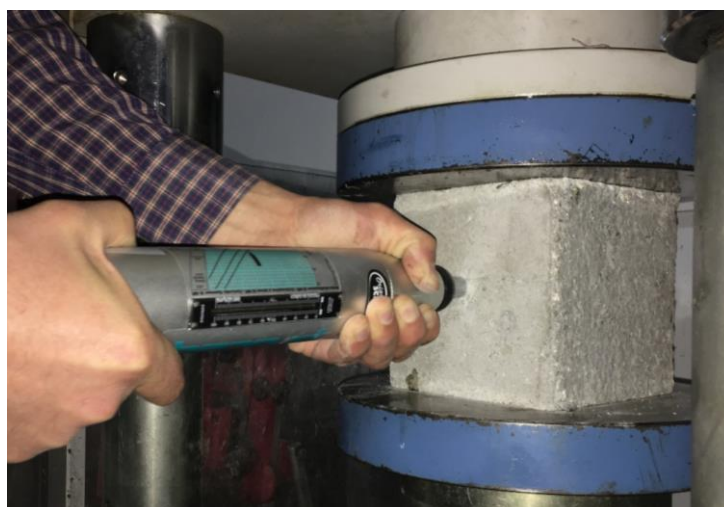
Fig. 5 - Schmidt Hammer test setup
