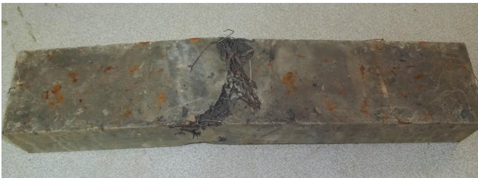
Fig. 8 - Fracture sample as a result of the flexural test
