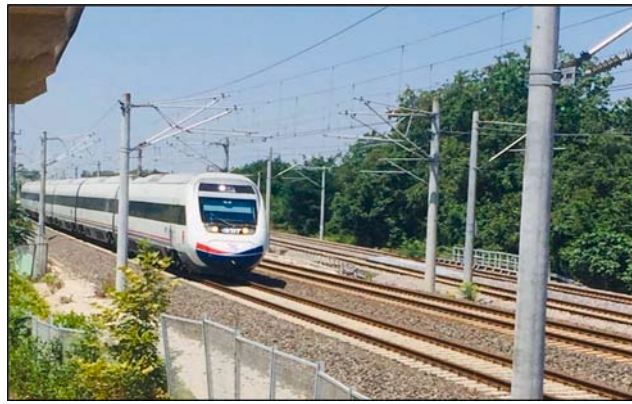
Fig. 5. Passage of the HT65000 high-speed train on Line 1 with speed V = 250 km/h (Kirkpinar, Sakarya 2018).
