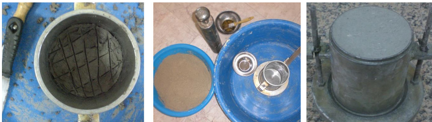
Figure 7. Standard compaction test specimen and phase of samples
