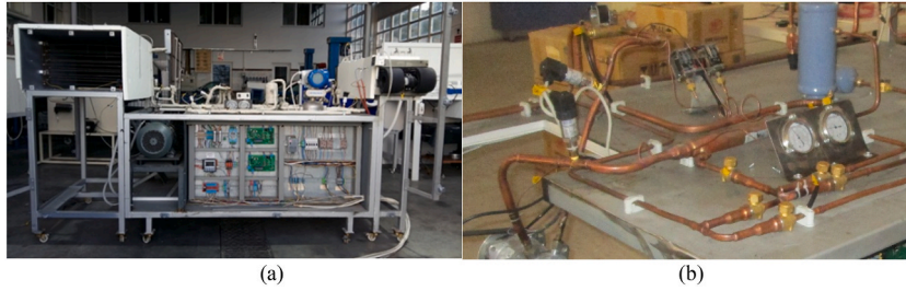
Fig. 2. Picture of the experimental AHP; (a) General view, (b) View of the SLHX assembly.
