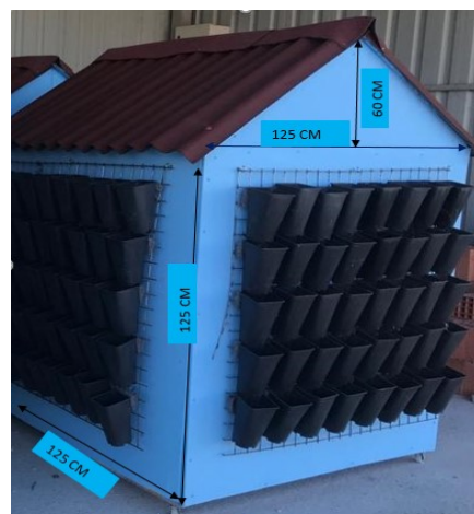
Figure 1. Construction of model buildings and the green wall system.
