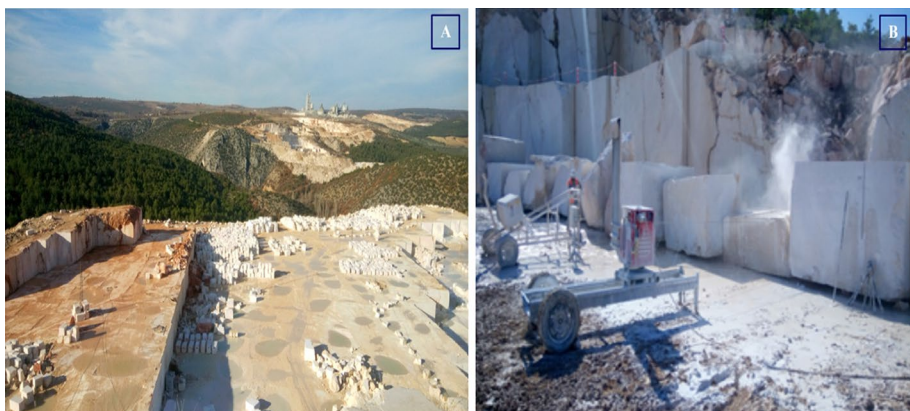
Fig. 1 a, b Open marble mine and cutting of marble blocks
