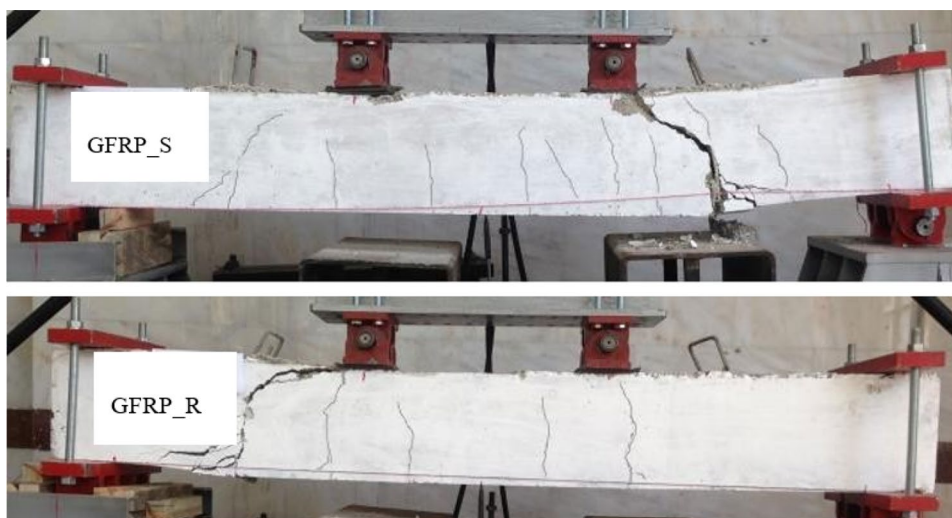
Fig. 14 Deformations of GFRP_S and GFRP_R-reinforced beams after flexural test
