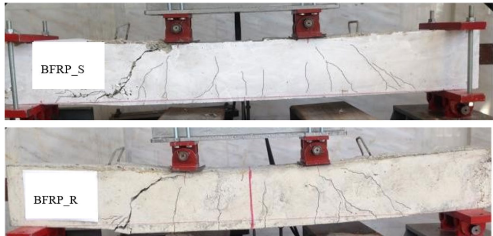
Fig. 10 BFRP_S and BFRP_R-reinforced beam deformations after flexural test
