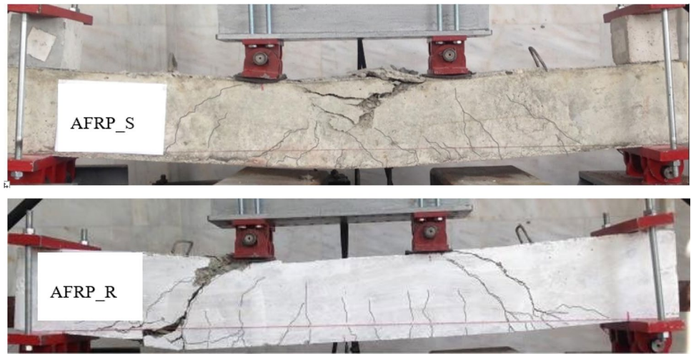
Fig. 8 Deformations of AFRP_S and AFRP_R-reinforced beams after flexural test
