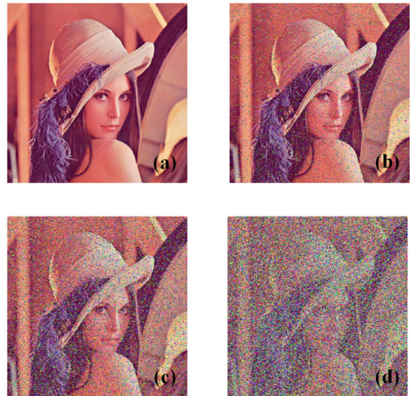
FIGURE 22. Decrypted image disturbed by salt-and-pepper noise: (a) noise density n = 0 , (b) noise density n = 0.05 , (c) noise density n = 0.1 , (d) noise density n = 0.2 .
