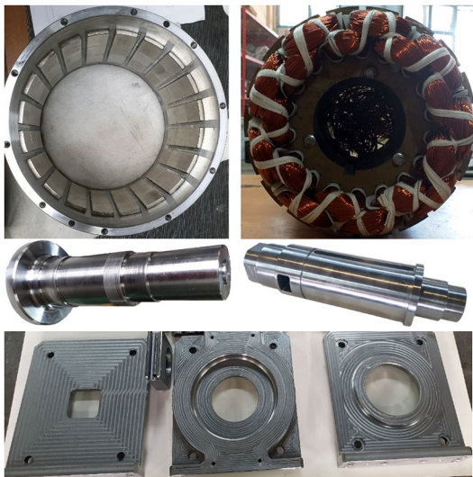
Fig. 14 Prototype parts of the elevator machine
