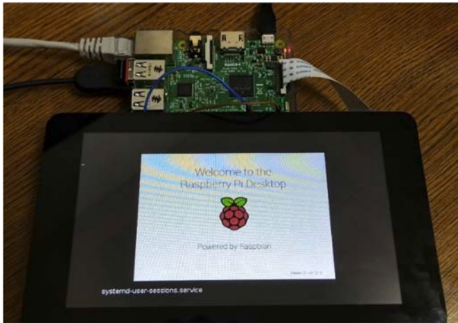
Fig. 8. Raspberry pi 3 model B desktop access.
