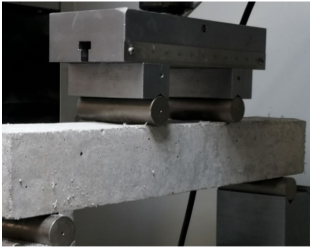
Fig. 5 Four-point bending test setup
