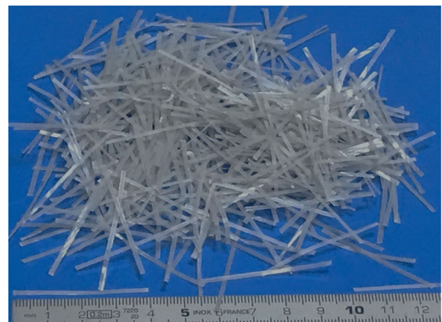
Fig. 3 Macro-synthetic fiber (KraTos Macro 40)
