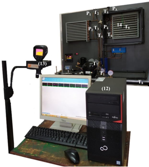
Fig. 3 Image acquisition from the experimental rig with a thermal camera
